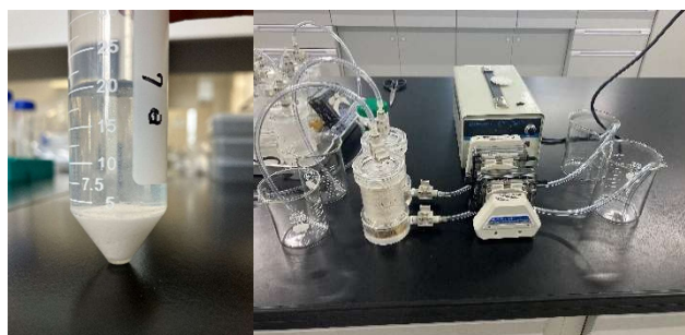
Fig.1 Batch test and soil column curing test
